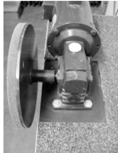
Below: Gearhead and motor mounted to a bench.
