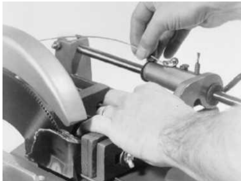
3. Gravity feed and vise are removed. Once this is done, slabs can be held by hand to be trimmed to desired shape.
