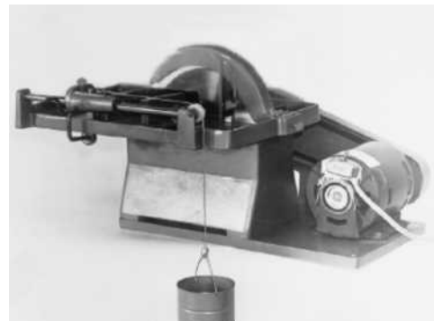
2. A bucket of sand is attached to the gravity feed cable to maintain an even pressure throughout.
