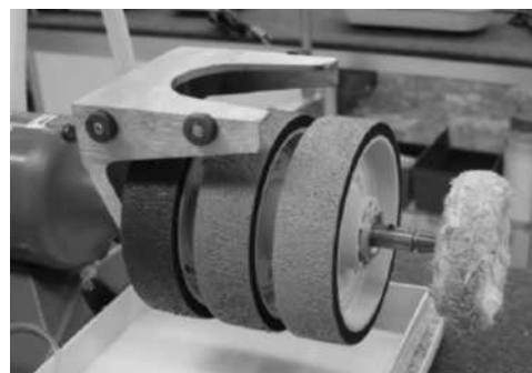
Shown on Genie: adaptor, tapered spindle and buff.
